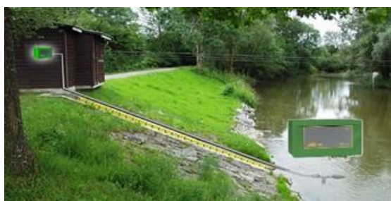
Bubble level sensor OTT CBS assembly
