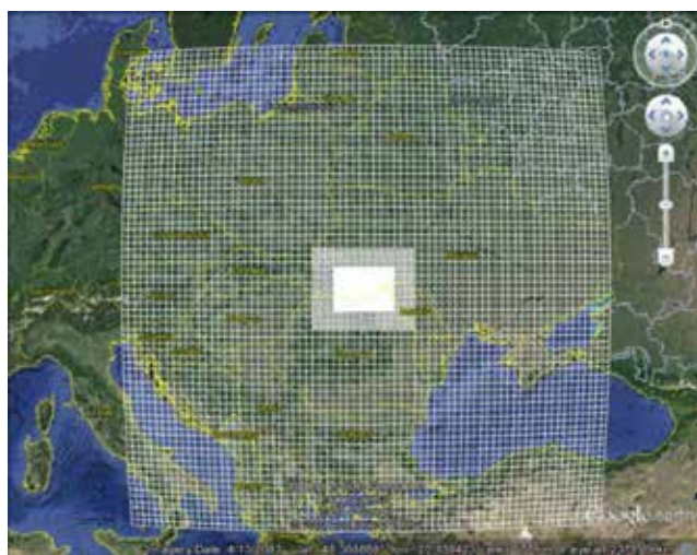
Three nested domains of the WRF model customized for the basins of the Prut and Siret rivers in Ukraine
