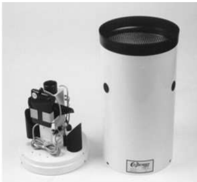
Pluviometer with tipping cups
