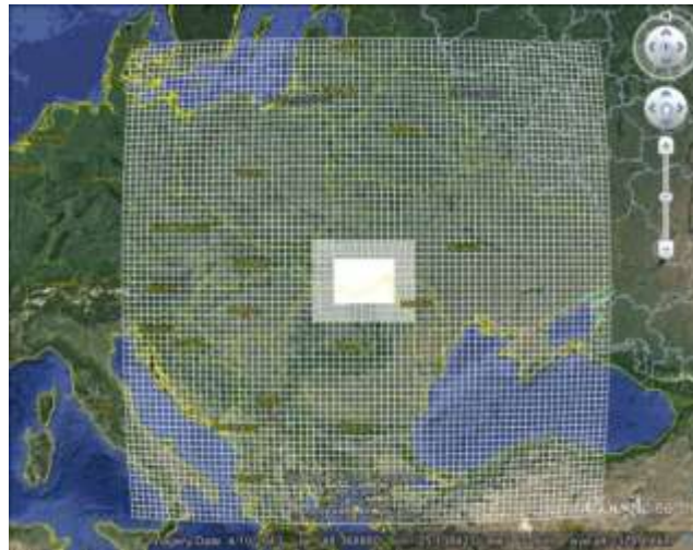
Figure 1 - Three nested domains of the WRF model customized for the basins of the Prut and Siret rivers in Ukraine.
