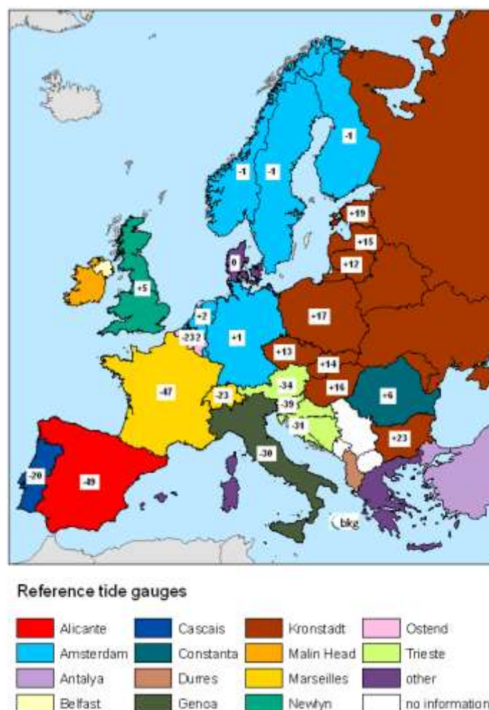
Fig. 3.3 - Mean differences between EVRF2007 and national height reference systems
