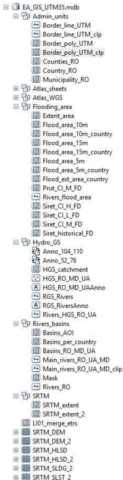
Fig. 7.13 – Initial structure of geodatabase for EastAvert project
