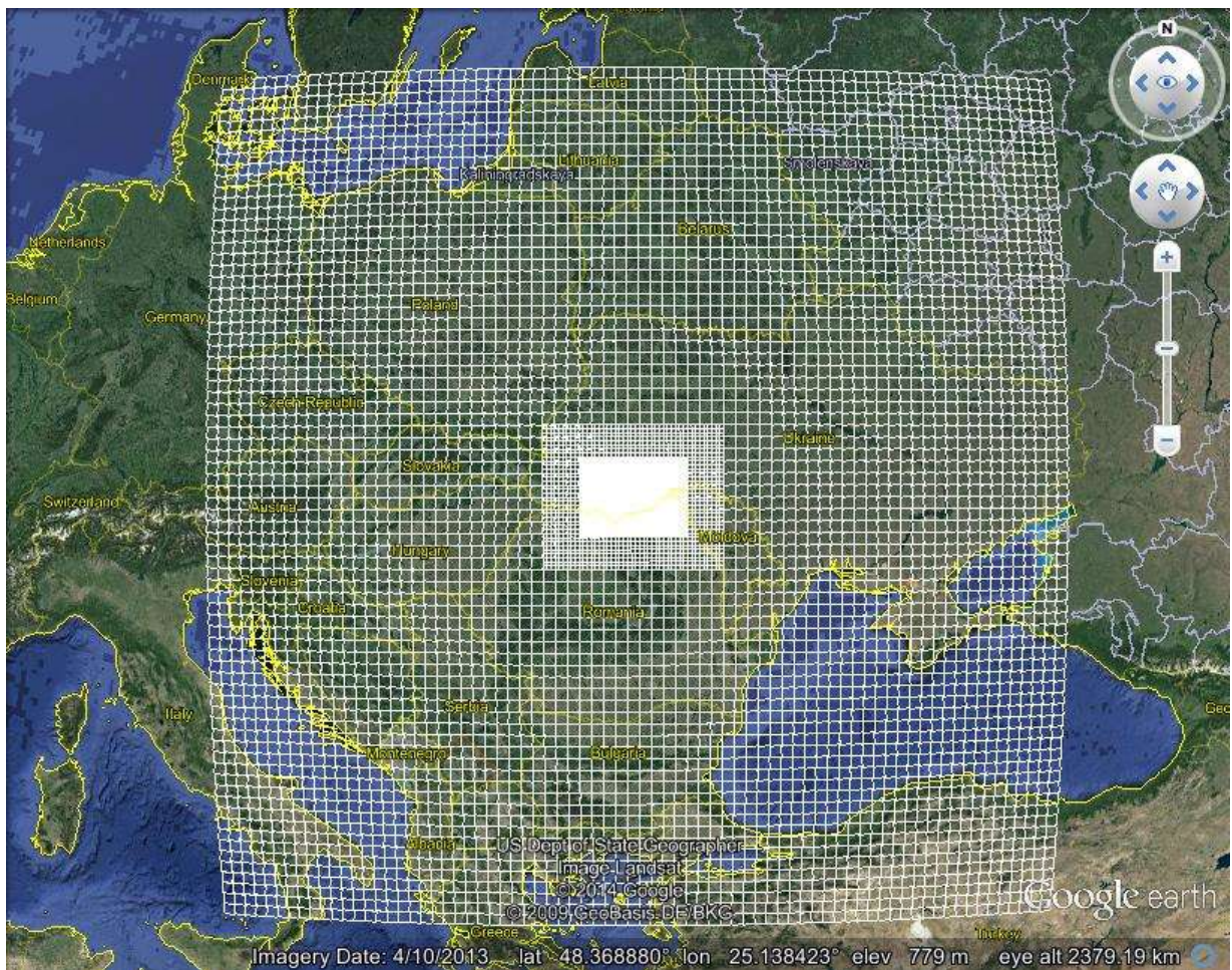
Fig. 1 Three nested domains of the WRF model customized for the basins of the Prut and Siter rivers in Ukraine
